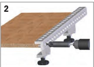
Place the jig onto the board, fix the end stop and tighten the workpiece. Set the bore depth and clamp the boring adapter on your drilling machine. Bore vertical holes.
