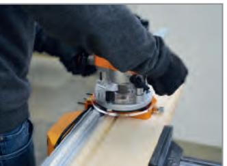
Holding onto your router in position, power on and begin making the cut by pushing forward and back on the straight edge clamp using the precision router dado jig as a guide. Makes impeccable grooves and dadoes along the length of your workpiece.
