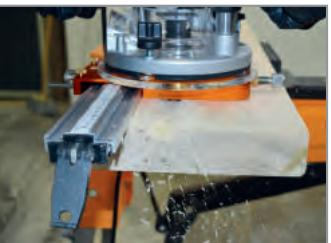
Set your cutting depth by raising or lowering the bit until desired depth is reached. Determine the starting point of the cut you wish to make by using the Dado Alignment Marks on the long sides (width) of the Adjustable Precision Router Dado Jig which indicates the outside edge of the dado cut closest to the straight edge clamp (12-10-8mm front, 1/2", 3/8", 1/4" back).
