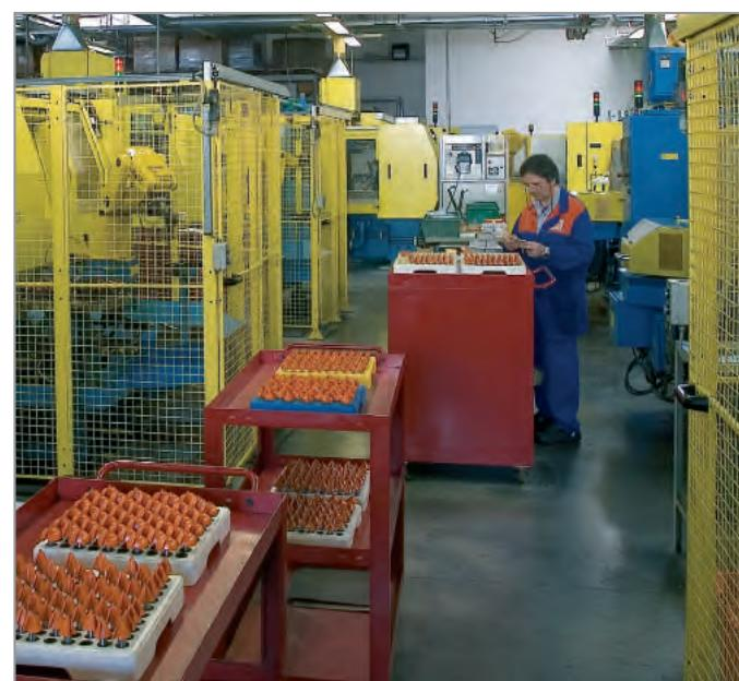
Loading the automated multi-axis CNC sharpening machines.
