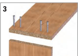
Now insert the dowels with glue into the holes and join both elements.
