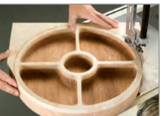
Bandsaw the exterior to final shape.
