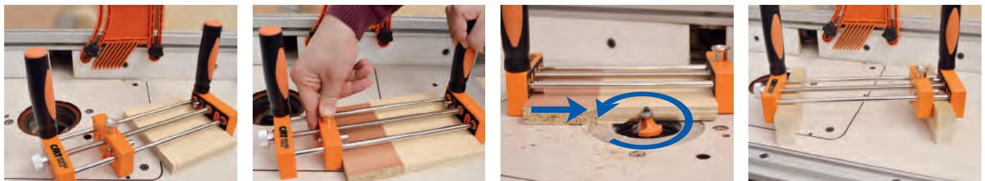
1. Lie the Small Stock Holder flat on the work surface. Slide the Hold Down Pins [F] to the top of the slotted holes. Insert the small stock piece between the Adjustable Centre [C] and Left-Side Bases [B]. The end of your small stock piece should lie flat and snugly up against the Left-Side Base. The end must also extend outwards in front of the Small Stock Holder a minimum distance of half the diameter of the router bit in use.
