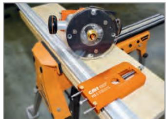
Prepare your router: Install the guide bushing rings into the bore baseplate and then attach it as the base for your router. Select and insert your router bit.
